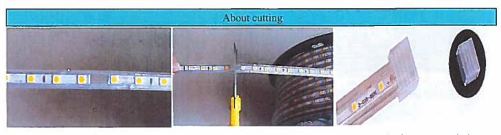
Find the transparent gap between the PCB and then cut the gap according to your required meters. And plug
