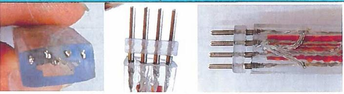
Important note: RGB LED Strip light have 4 cable inside and the space between each cable is small. Make sure that each cable will not touch together when plug the 4 pins into the led strip light. Otherwise will cause short circuit and damage the controller.
